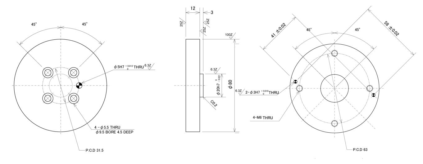
According to the diagram above, open mounting holes for the robot from the force sensor mounting side.
